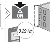
The result is shown in the main line and the measured distance above. Pressing the measuring key for 2 sec in the function activates automatically Minimum or Maximum measurement.
