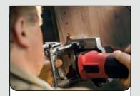
Rows of holes can be drilled quickly and accurately with the aid of the auxiliary stops, even in furniture that has already been assembled.
